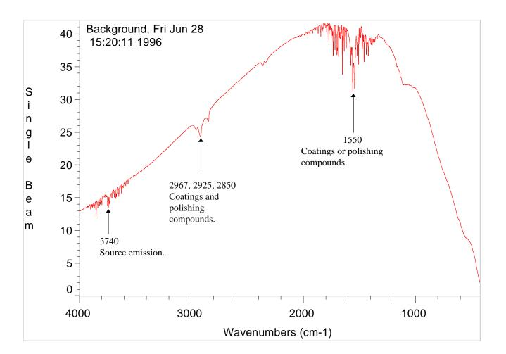
This is a typical single beam from an Impact with TGS detector. Because of the polishing compounds and the moisture protective coatings on the lenses, spectrum features show up in the following areas:
