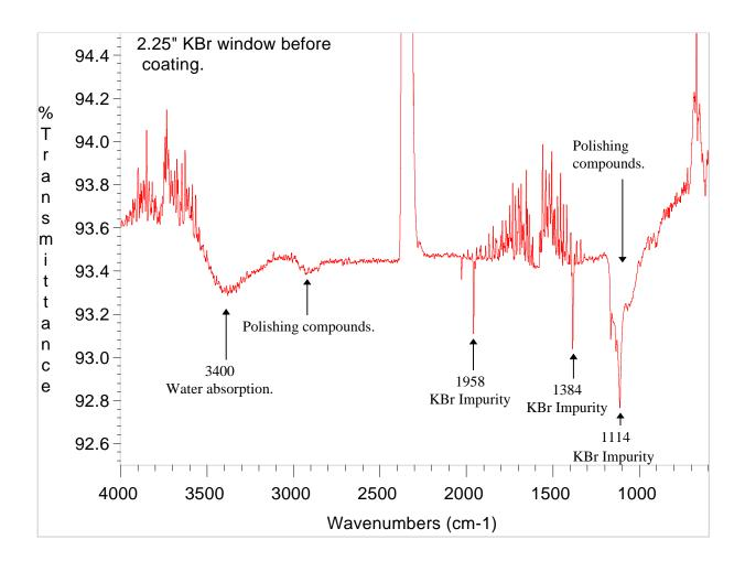
The plot above is a transmission spectrum of a 2.25" dia. KBr window before coating for moisture protection. This piece of KBr has more impurities than the coated KBr window example on page 2. There is also a wide band around 3400 wavenumbers from water absorption onto the KBr.
