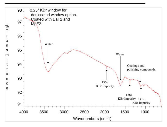
The plot above is a transmission spectrum of a coated KBr window. This example shows severe degradation from water absorption. This measurement was taken from a 2.25" dia. window used for the Magna desiccated option. This plot shows the wide areas of water absorption into the KBr and the coatings. Also, this shows the impurity bands in the KBr crystal.
